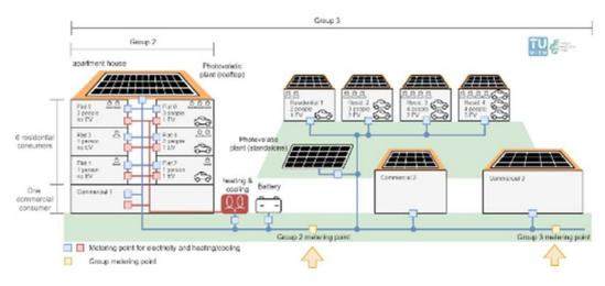
Figure 1 : Schematic of group 2 and 3 with group metering points
