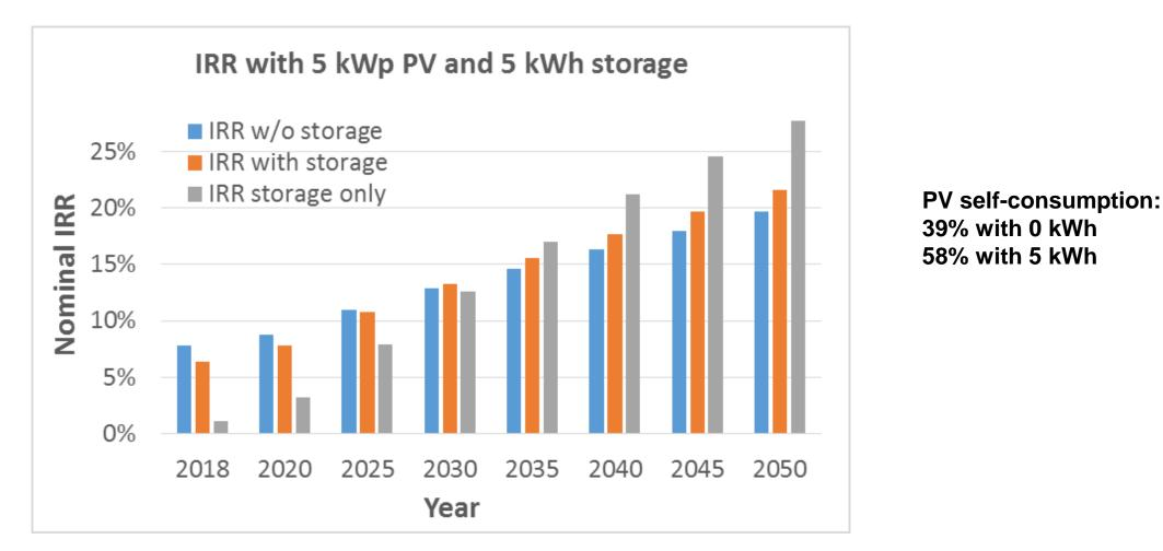
PV system size 5 kWp, usable storage capacity 80%, round-trip efficiency 90%, annual consumption 5 MWh PV CAPEX 1.2-0.55 €/Wp + VAT and OPEX 19-11 €/kWp/a, storage CAPEX 600-130 €/kWh + VAT and OPEX 6-3 €/kWh/a PV yield 1040 kWh/kWp, annual degradation 0.5%, PV system lifetime 30 a, storage system lifetime 15 a Annual inflation 2%
