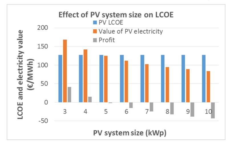
PV self-consumption: 57% with 3 kWp 22% with 10 kWp
