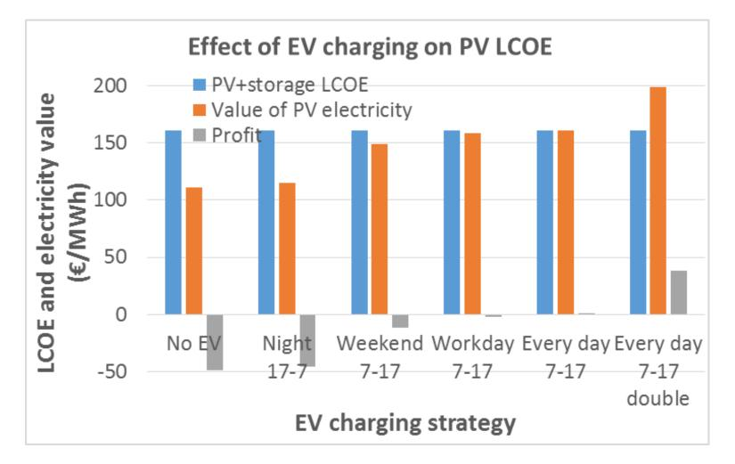
PV system size 10 kWp, battery system 5 kWh, usable storage capacity 80%, round-trip efficiency 90%, PV CAPEX 1.2 €/Wp + VAT and OPEX 19 €/kWp/a, storage CAPEX 600 €/kWh + VAT and OPEX 6 €/kWh/a PV yield 1040 kWh/kWp, annual degradation 0.5%, PV system lifetime 30 a, storage system lifetime 15 a Nominal WACC 8%, annual inflation 2%; annual consumption 5 MWh
