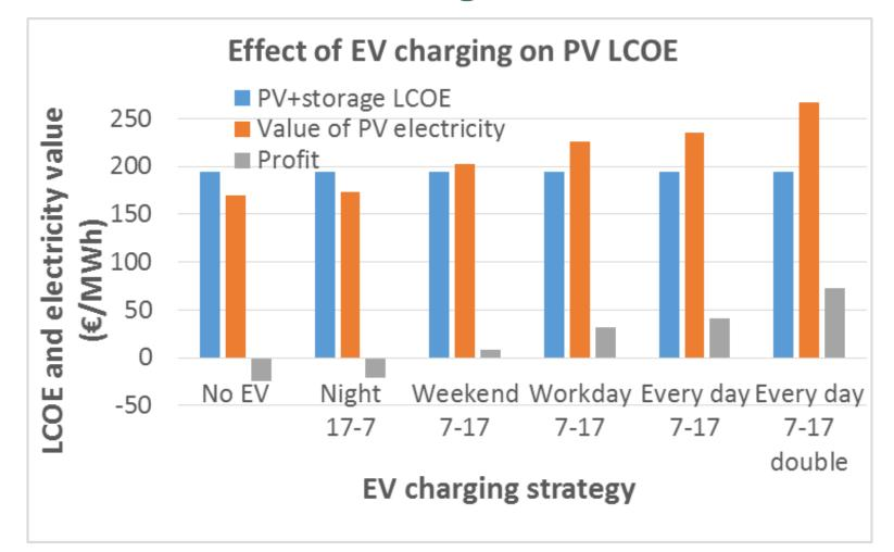
PV system size 5 kWp, battery system 5 kWh, usable storage capacity 80%, round-trip efficiency 90%, PV CAPEX 1.2 €/Wp + VAT and OPEX 19 €/kWp/a, storage CAPEX 600 €/kWh + VAT and OPEX 6 €/kWh/a PV yield 1040 kWh/kWp, annual degradation 0.5%, PV system lifetime 30 a, storage system lifetime 15 a Nominal WACC 8%, annual inflation 2%; annual consumption 5 MWh
